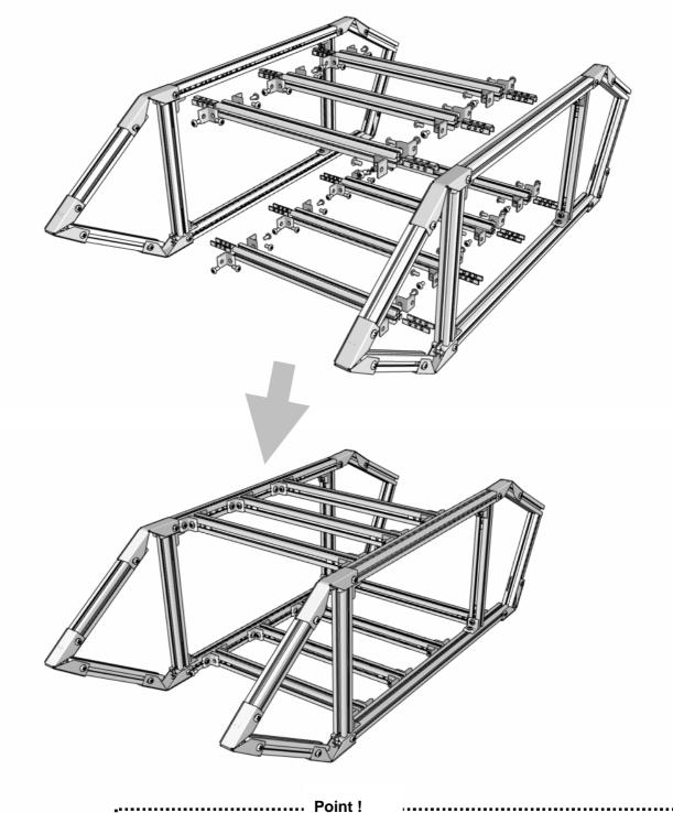
Insert metal slides into 256mm frame (3 pcs above) used for connecting side surface of vehicle beforehand in order to mount top part and battery. Mounting motherboard will be done easily by placing an extra metal slide into 256mm frame (4 pcs below) used for connecting side surface of vehicle. Refer to Basic Assembly< Fixing Motherboard>.  Mounting power supply fixing frames Mount 256mm frame for fixing power supply.
