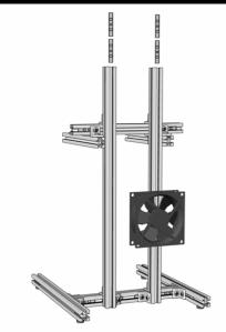
Drill 2 Sliders (3S) into the back of the pillar. Attach the 8cmFAN to the height of your choice.
